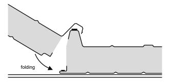
The follow-up panel is to be positioned alongside the high rib of the panel installed preliminarily and then let down onto the construction. This way, you make sure that the joint is sealed and no visible offset appears on the internal side.
