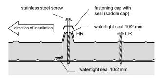
A static engineer must determine how many screws are needed for the surface, the corners and edge areas.
