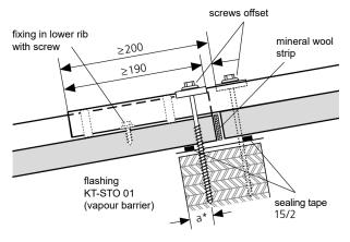
\* distance to edge when using wooden purlin a ≥ 5 x screw diameter (compare DIN 1052, part 1)
