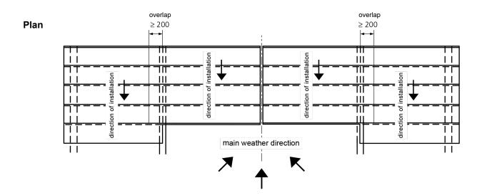
With roof lengths longer than the max. shipping lengths or heavier than the max assembly weight, panels are to be adjusted successively. They are fastened with an overlapping joint.
